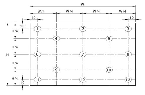
Note 3: The luminance uniformity of 5 or 13 points is defined by dividing the maximum luminance values by the minimum test point luminance
